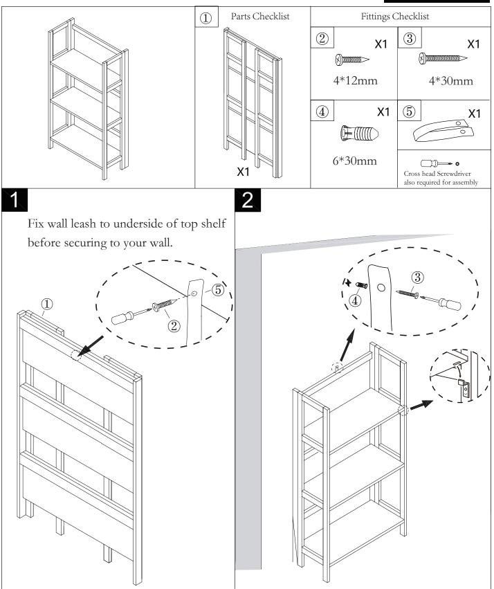
A wall leash is recommended for this product. Before moving the shelf into place, establish the correct height to attach the 'wall leash' to the wall. Wall leash fittings supplied are standard, different wall types may require fixings that are suitable for your wall type. Contact your local specialised hardware store for advice on suitable fixing.
