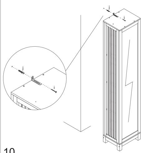
Follow this step to fix your Shoe Tower to the wall. Fixing to secure your Shoe Tower to the wall is standard fitting. For details on suitable fixing for your wall type seek advice from your local specialised hardware store.
