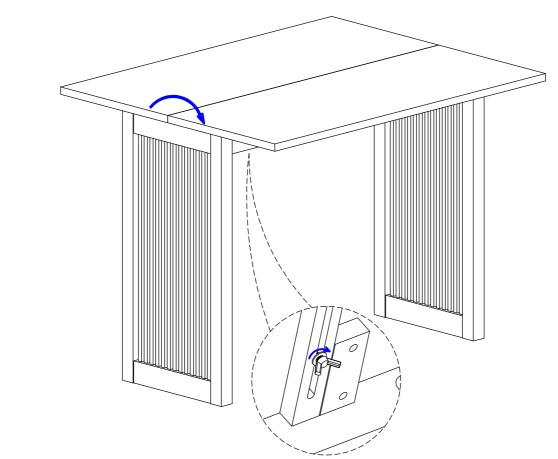
**8.** Fold open leaf and tighten slide lock.
