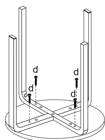
Fitting D fixes into outer hole.
