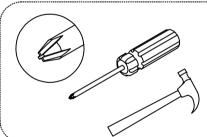
You will need a cross head screwdriver and a hammer to assemble this product. An electric drill may cause damage and is not recommended.
