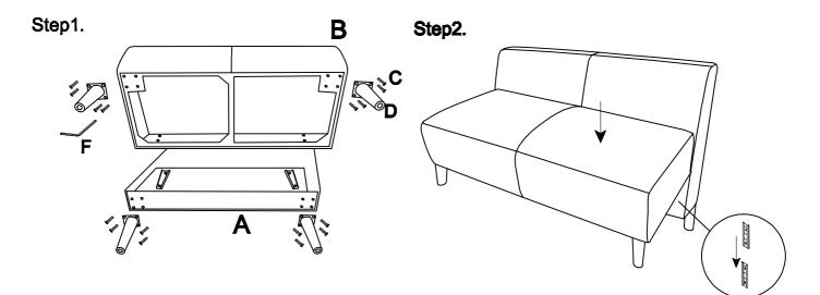
After assembling the legs, push the seat down onto the backrest. Then, sit on the sofa firmly BEFORE fixing the four bolts part E.
