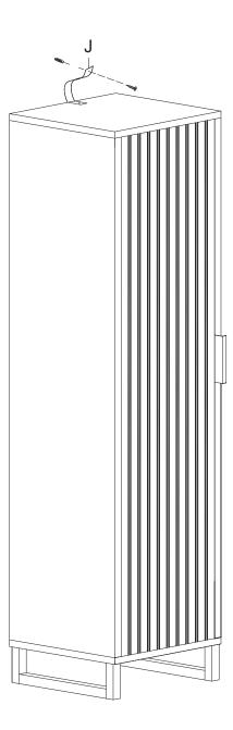
Fitting J should be used to secure your ST CALX TOWER to the wall. Screws and fittings for wall are not supplied as different wall constructions require fittings that are suitable for your wall type. If you are unsure for the correct type of fitting for your wall, please contact your local specialised hardware store for information on suitable fitting.
