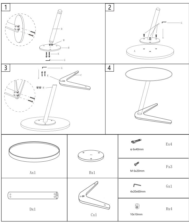
During assembly steps do not fully tighten fittings. Tighten to 80%. This will allow for easier assembly of all parts, then in final step tighten all fittings fully before using your table.
