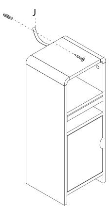
Fitting J should be used to secure your ST CAB HALE to the wall. Screws and fittings for wall are not supplied as different wall constructions require fittings that are suitable for your wall type. If you are unsure for the correct type of fitting for your wall, please contact your local specialised hardware store for information on suitable fitting.
