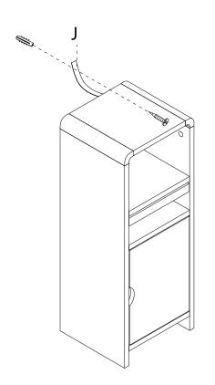
Fitting J should be used to secure your ST CAB HALE to the wall. Screws and fittings for wall are not supplied as different wall constructions require fittings that are suitable for your wall type. If you are unsure for the correct type of fitting for your wall, please contact your local specialised hardware store for information on suitable fitting.
